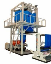
Two Layer Haul off Attachment HMHDPE / LDPE/LDPE Blown Film Plant
