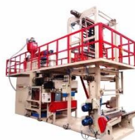
Polypropylene / LDPE / LLDPE Film Plant with Opening Attachment
