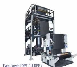
Two Layer LDPE / LLDPE / Mulching Blown Film Plant
