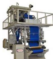
Multi Layer A-B-C Blown Film Plant with haul off attachment
