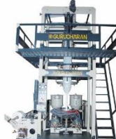
Two Layer with Three Layer (A+B+A) & (A+B) Single Die Head HMHDPE Blown Film Extruder
